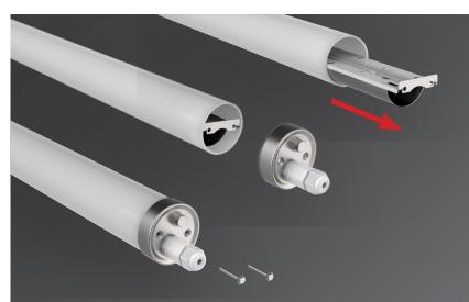
Repairable design: by removing the screws and the end cap, the gear tray can be slid out of the luminaire allowing for repair, without losing the IP69K protection of the product.
