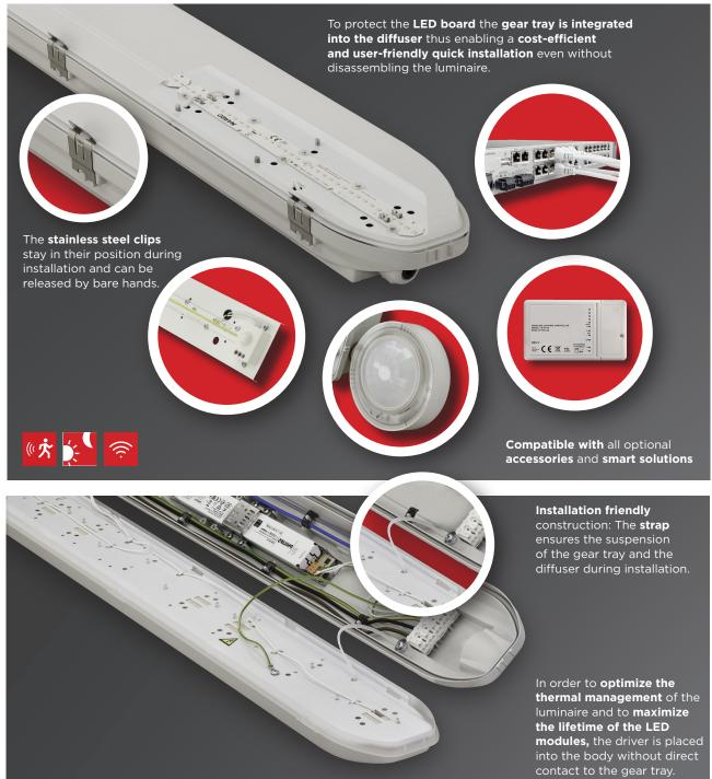
The gear tray, made of white powder coated steel sheet according to Zhaga standards, is integrated into the diffuser. With 870-Inspire GRP - depending on customer requirements - we can reach different levels of luminous flux from 2700 up to 14000 lumen and a maximum efficacy of 160 lm/W. Details see: For more details please see technical data.
