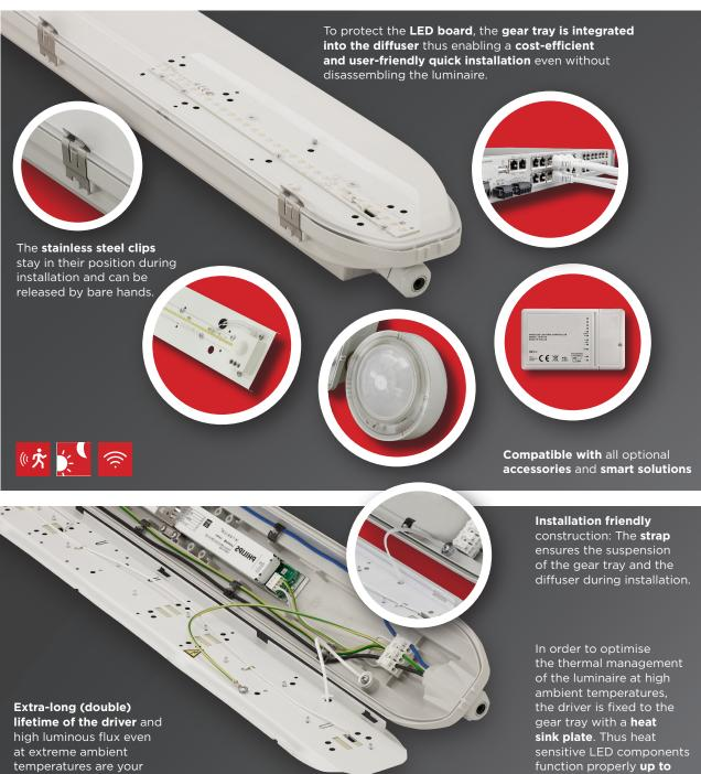
The gear tray, made of white powder coated steel sheet according to Zhaga standards, is integrated into the diffuser. With 870-Inspire +/- - depending on customer requirements - we can reach different levels of luminous flux up to 10400 Im and a maximum efficiency of 153 Im/W. For more details please see technical data.
