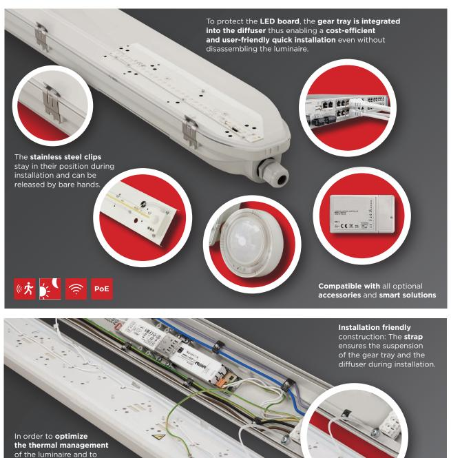
The gear tray, made of white powder coated steel sheet according to Zhaga standards, is integrated into the diffuser. With 870-Inspire PC - depending on customer requirements - we can reach different levels of luminous flux from 3000 up to 12900 lumen with maximum efficacy of 152 lm/W. For more details please see technical data.
