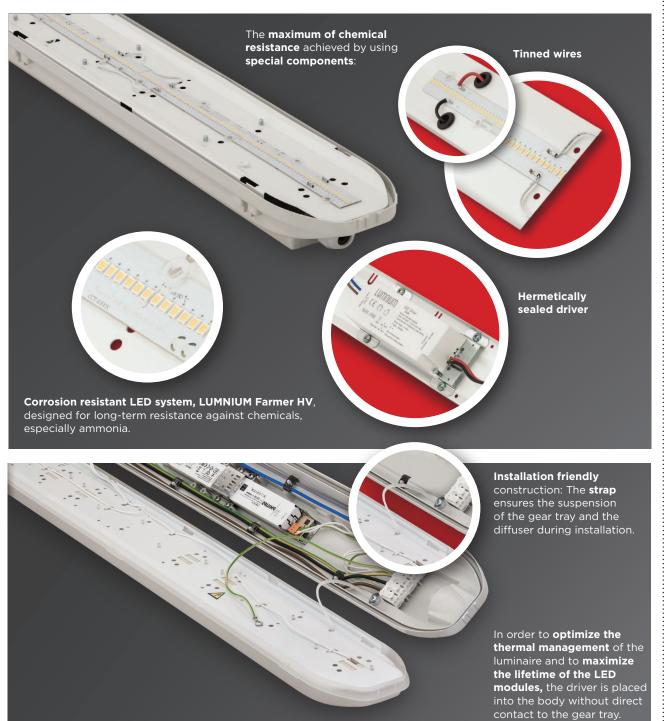
The **gear tray**, made of white powder coated steel sheet according to **Zhaga** standards, is **integrated into the diffuser**. With 870-Farmer - depending on customer requirements - we can reach different levels of luminous flux from 3800 **up to 6600 lumen** with maximum **efficacy of 164 lm/W**. For more details please see technical data.
