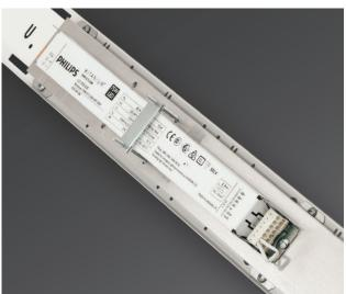
In order to optimise the thermal management of the luminaire at high ambient temperatures, the driver is fixated to the gear tray with a heat sink plate. Thus heat sensitive LED components function properly up to Ta +50°C.
