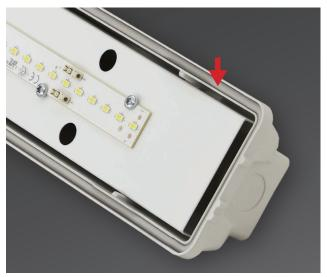
In order to ensure maximum heat, chemical and weather resistance even under tough conditions, the gasket between the diffuser and housing is made of silicone-based foam with enhanced resistance.
