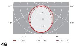
771-Extreme -30°C 4ft (2x1500mm) Philips Fortimo LED HV6, 70W, 9900lm, PC
